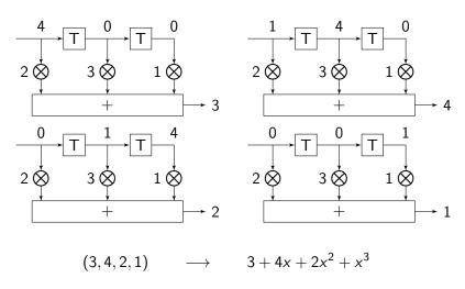
The Linear Feedback Shift Register architecture for division by  $3 + 2x + x^2$  over GF(5). Preparation: the coefficients are
