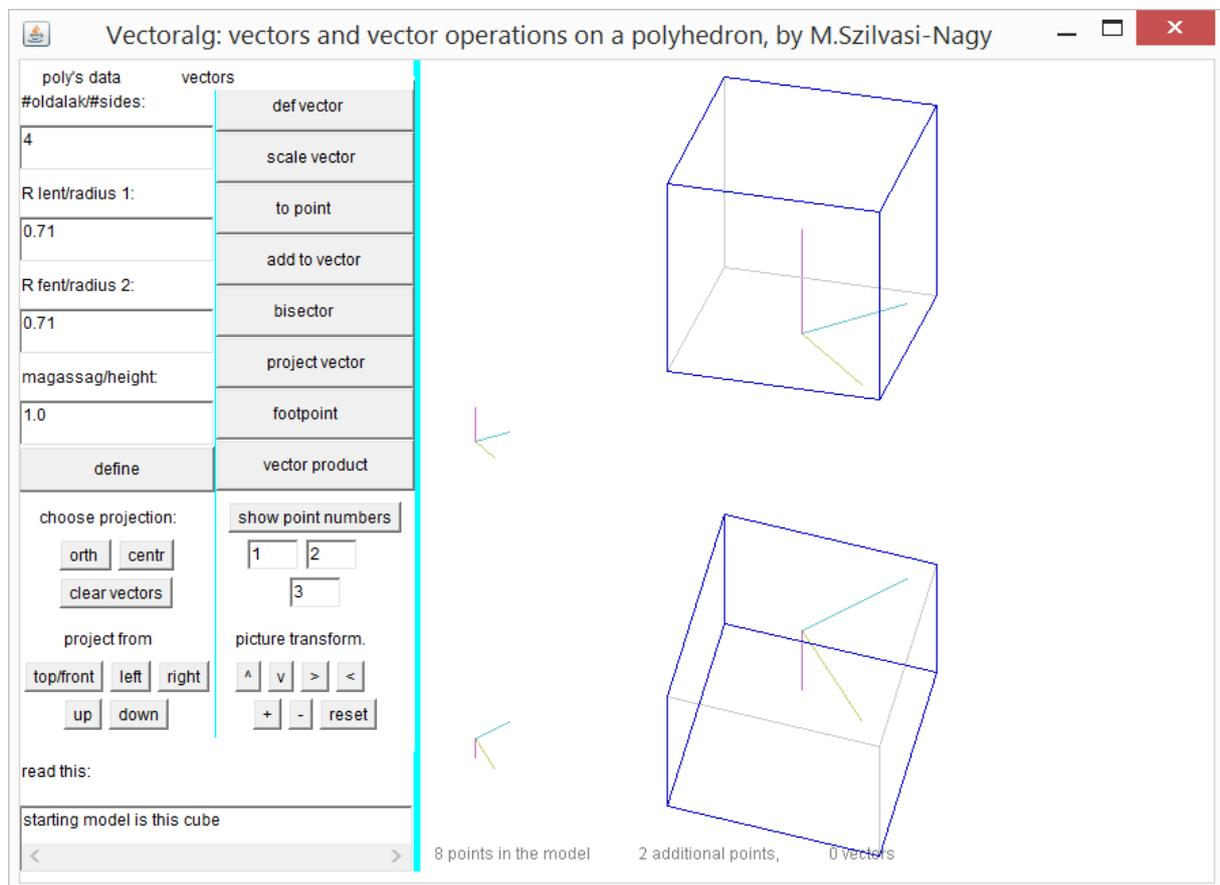
**The polyhedron** is a regular truncated pyramid defined by the number  $n$  of side faces, the radius  $R_1$
